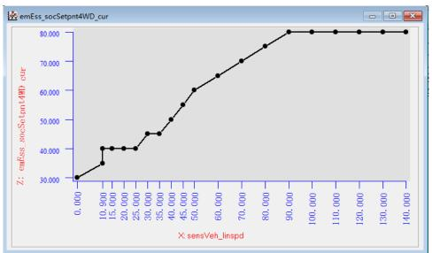
'2D View' window also support **graphical based calibration**. You can use mouse to drag one of the points to revise calibration value.
